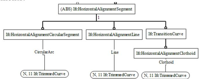
Figure 5. Horizontal alignment segments use and *IfcTrimmedCurve* (part of standard IFC 4) to describe its geometry
