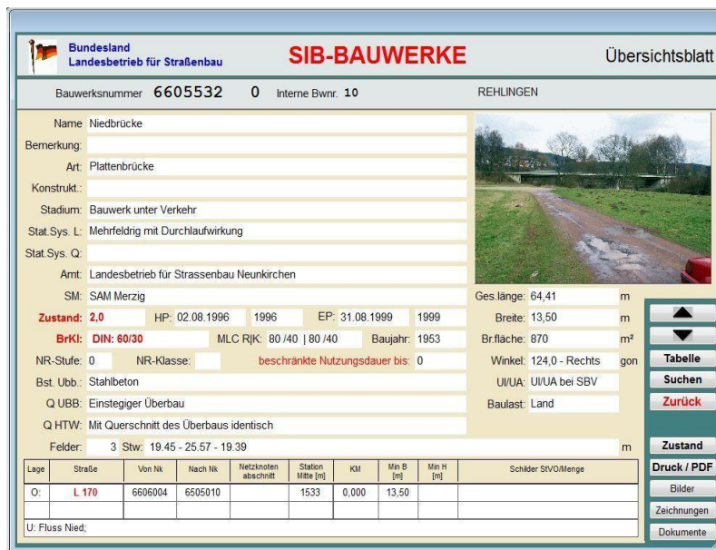
Figure 2: General view in the bridge management system SIB-Bauwerke (WPM - Ingenieure 2015)
