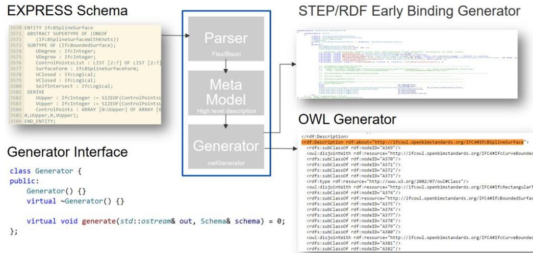
**Figure 2. IFC Tunnel EXPRESS Schema conversion to OWL**
