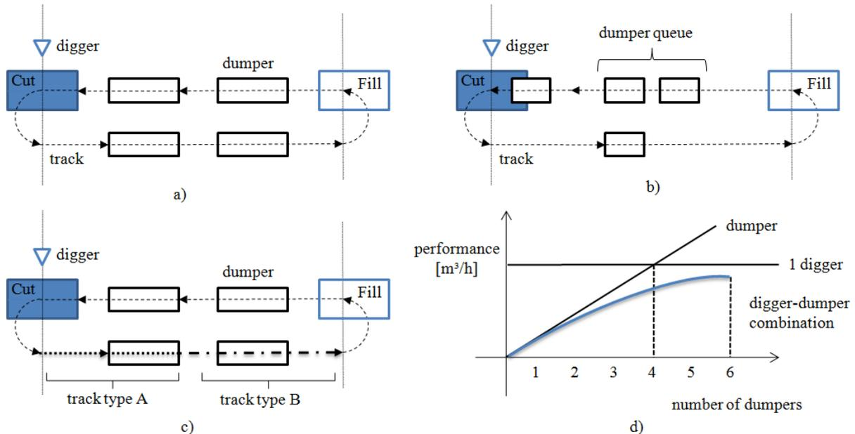
Figure 1: Detailed modeling of earthwork processes under consideration of microscopic conditions; a) ideal process b) waiting queue c) properties of tracks d) non-linear working performance in earthwork processes
