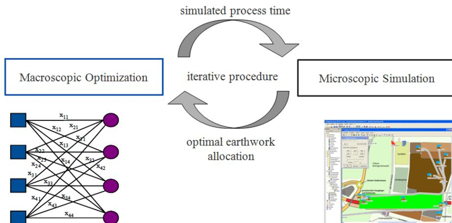
Figure 2: Principle of the iterative method coupling microscopic simulation and macroscopic optimization
