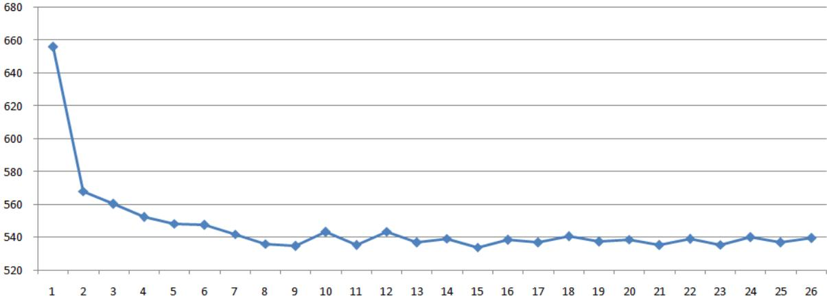
Figure 5: Changes of total earthwork process time [h] (vertical direction) during 26 iteration steps (horizontal direction)
