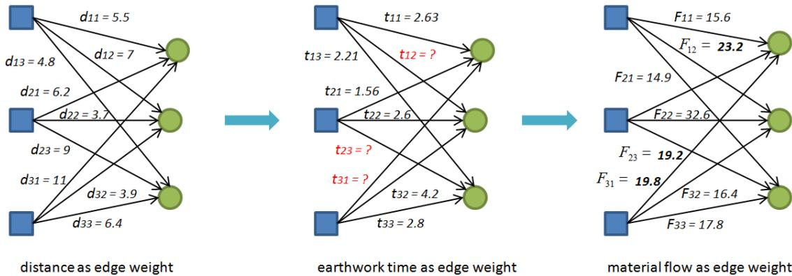
Figure 4: Converting the earthwork process time in material flow for each cut-to-fill pair
